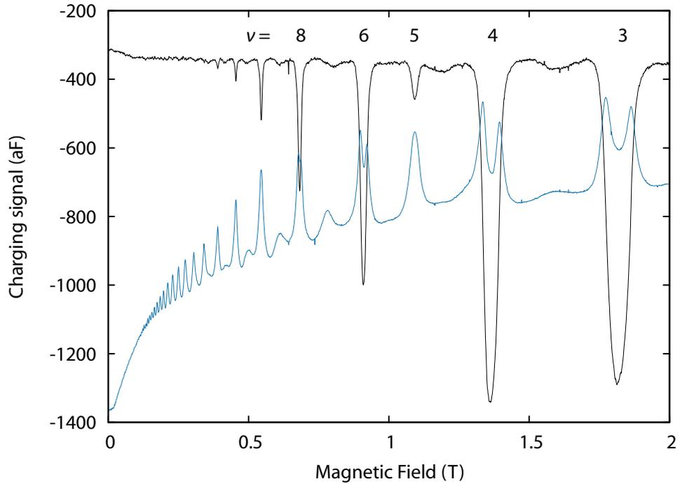
Figure 2-18: A high mobility sample (wafer 12-16-03.2) showing charging signal oscillations down to very low magnetic fields. Oscillations at even filling factors are seen up to Landau level index  $>40$  in the lagging phase.
