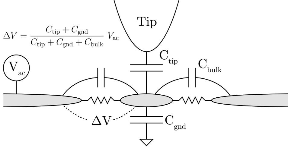
Figure 2-10: Model of an island in the 2D electron system that is isolated from the bulk by a resistive ring. In the high resistance limit  $R \gg 1/\omega C$ , there will be a voltage drop  $\Delta V$  across the ring given by  $V_{\text{ac}}$  divided by a capacitive “lever arm”. This lever arm factor is given by the ratio of the island’s capacitance to ground and the tip to its self capacitance.
