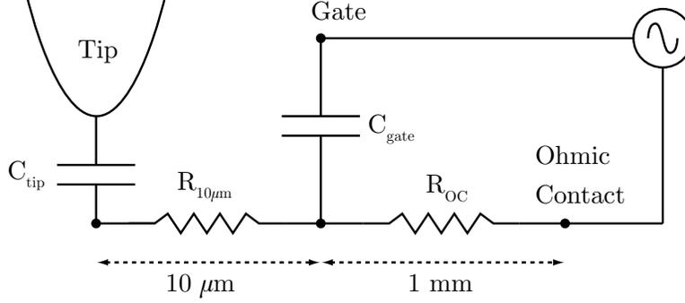
Figure 2-16: Schematic illustration of charging of the 2D layer in a sample with a topgate. At Hall plateaus, the resistance to the ohmic contact  $R_{\text{OC}}$  diverges. The presence of the gate allows us to still drive AC charge onto the tip capacitor through the capacitive coupling of the gate to the 2D layer.
