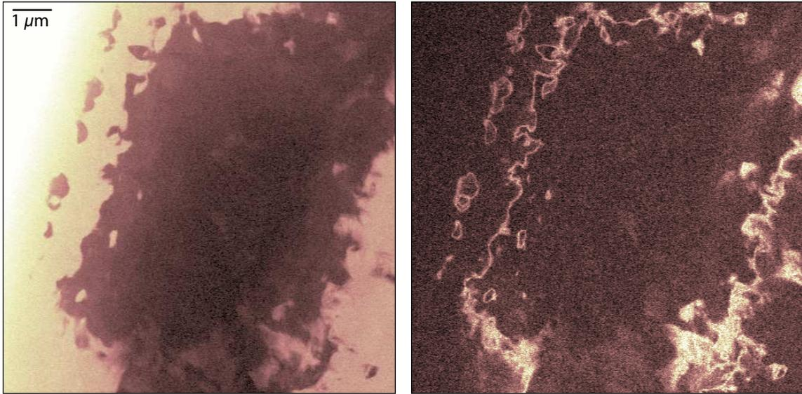
Figure C-6:  $10 \times 10 \mu\text{m}$  in-phase and lagging phase images at 6.4T and 0.25V (near null) with a 5 mV excitation. Features in the image are far sharper than we expect from the electrostatic resolution of the tip determined from the smearing of the gate edge. Similar over-sharp features were seen using an etched tip that had not touched the surface.
