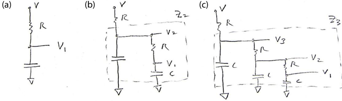
Figure E-1: Schematics for (a) 1 element RC network, (b) 2 element RC network, and (c) 3 element RC network.
