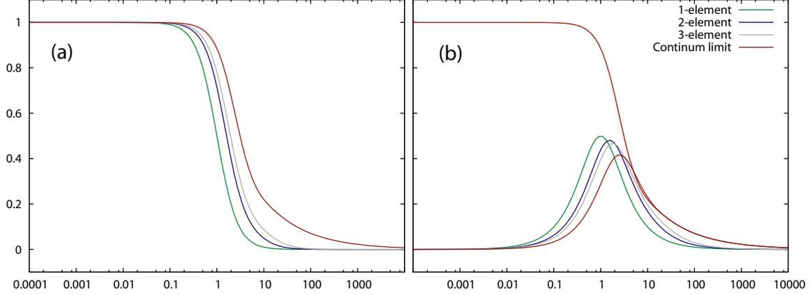
Figure E-2: In-phase (a) and lagging-phase (b) components of the total charge on the capacitors. In the discrete element models, elements were chosen so that  $\sum C = 1$  and  $\sum R = 1$ . In the continuum model, we took  $\epsilon L^2 / \sigma_{xx} d = 1$ . In (b), the real component was also plotted for the continuum model. This is to demonstrate the interesting fact that in the high frequency limit of this model, the two curves show the same asymptotic behavior.
