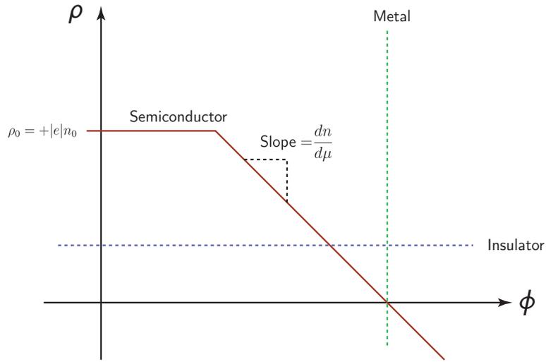
Figure 5-3:  $\rho(\phi)$  for a metal (green dashed line), an insulator (blue dashed line) and a semiconductor (red line). Due to the finite density of states, the curve for a semiconductor has a finite slope. A semiconductor with a fixed density of negative carriers  $n_0$  will have a maximum possible space charge density of  $\rho_0 = +|e|n_0$ , corresponding to full depletion.
