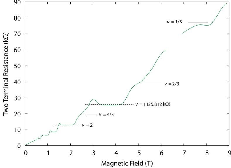
Figure 4-10: Two terminal magnetoresistance of the sample taken on the first cooldown before illumination. The  $\nu = 1$  plateau occurs at the same position as the signal from the bulk charging in the magnetocapacitance trace. Weak plateaus from some fractional states are also seen. The measurement was taken at a current bias of 100 nA. (The lock-in amplifier went off scale during the measurement at the positions of the missing data points.)
