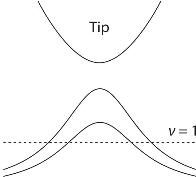
Figure 3-20: Applying a larger DC voltage to the tip does not necessarily increase the density gradient at the position of the strip because the point where the density crosses  $\nu = 1$  also moves out to a larger radial position. For this example, we show two Lorentzian density profiles, one of which corresponds to a larger tip voltage than the other by a factor of 1.5.
