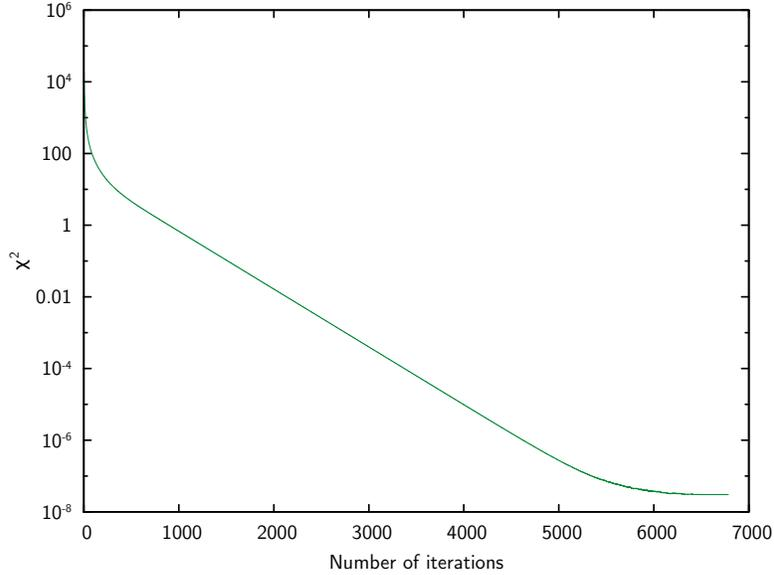
Figure 5-1: A plot of the average squared residual error as a function of the number of relaxations for simple relaxation.  $\chi^2$  shows an initial rapid drop as the values of the potential diffuse in from the boundaries. The long tail is associated with the slow damping of long wavelength error in  $\phi$ .
