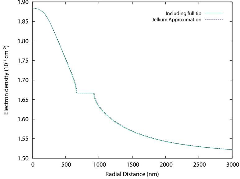
Figure 5-15: Comparing the electron density profile at  $\nu = 0.8$  calculated using the full tip (solid green line) to the calculation using the “jellium” approximation to reproduce the density profile from the tip (blue dashed line).
