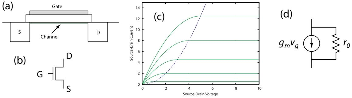
Figure B-1: (a) The layout of a typical field effect transistor and (b) the schematic symbol used. (c) I-V curves for an ideal FET. The dotted line shows the saturation current for the quadratic model. (d) A common model of a FET using a current source in parallel with an output resistance.
