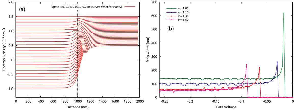
Figure 5-13: (a) Density profile as a function of topgate voltage at  $\nu = 1.2$ . The dashed line indicates the position of the gate on the surface of the sample. (b) Calculated strip width at a function bias voltage for different magnetic fields corresponding to the indicated bulk filling factor. After the initial formation, the strip width is independent of the the bias voltage.
