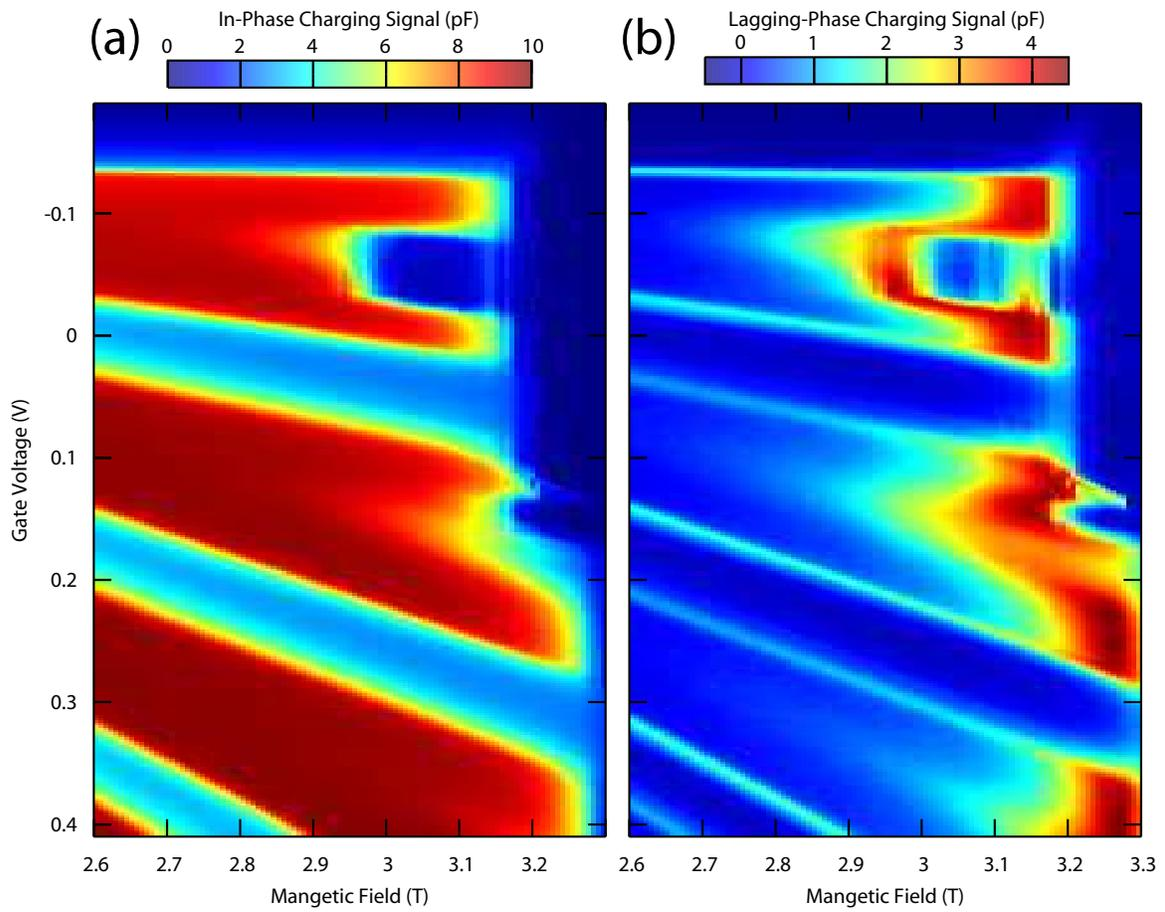
Figure 4-7: In-phase (a) and lagging-phase (b) charging data taken near the low field side of  $\nu_{\text{bulk}} = 1$ . Near the edge of  $\nu_{\text{bulk}} = 1$ , the charging signal is suppressed at low densities, but then recovers at higher gate voltages. There is also a strong resistive suppression of the signal at lower magnetic fields at biases that are close to  $\nu_{\text{local}} = 1$ .
