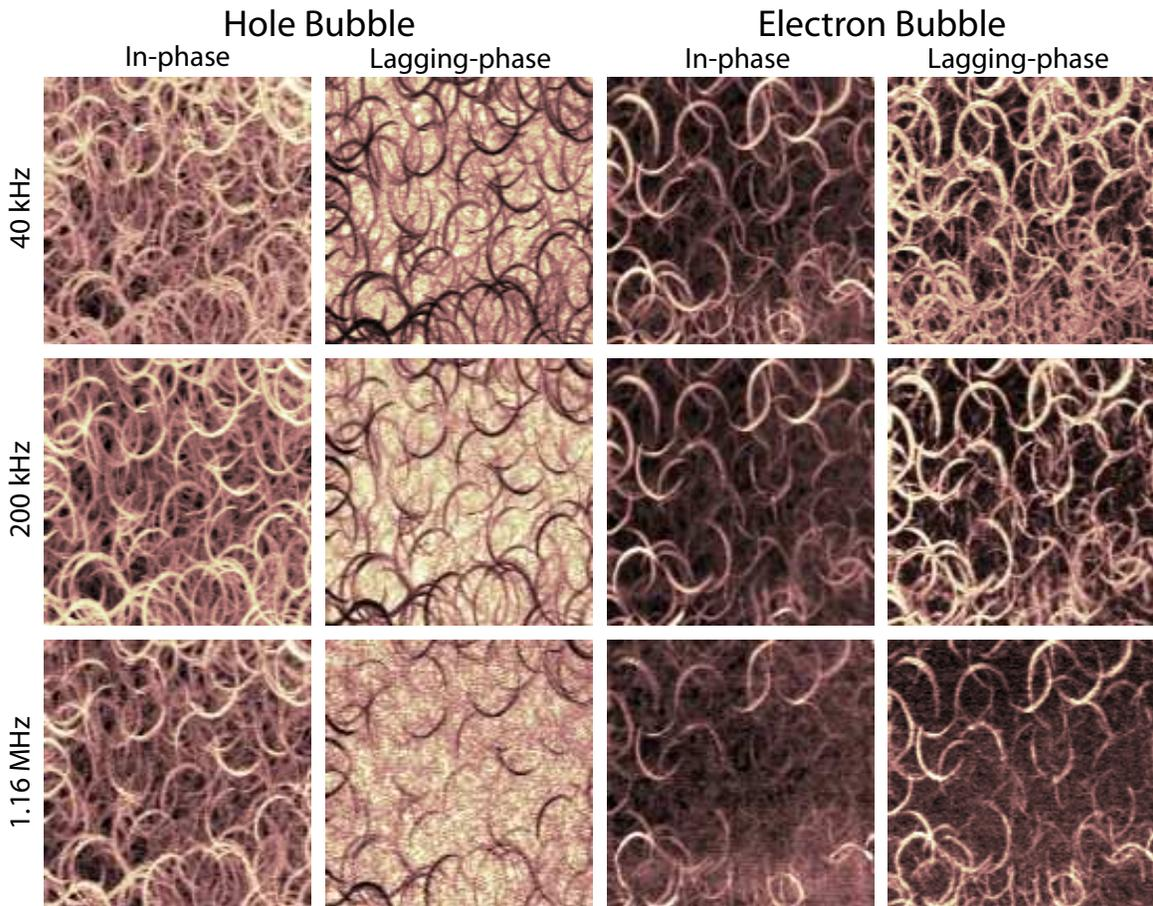
Figure 3-13: Frequency dependence of the resonance images at  $\nu = 1$ . The left two panels show  $9 \times 9 \mu\text{m}$  in-phase and lagging-phase hole-bubble images taken at 5.0T ( $\nu = 1.26$ ) at +1.75V. Images were taken at 40 kHz, 200 kHz, and 1.16 MHz. The right panel shows the same measurements for an electron bubble at 7.5T ( $\nu = 0.83$ ) with a tip bias of -1.75V.
