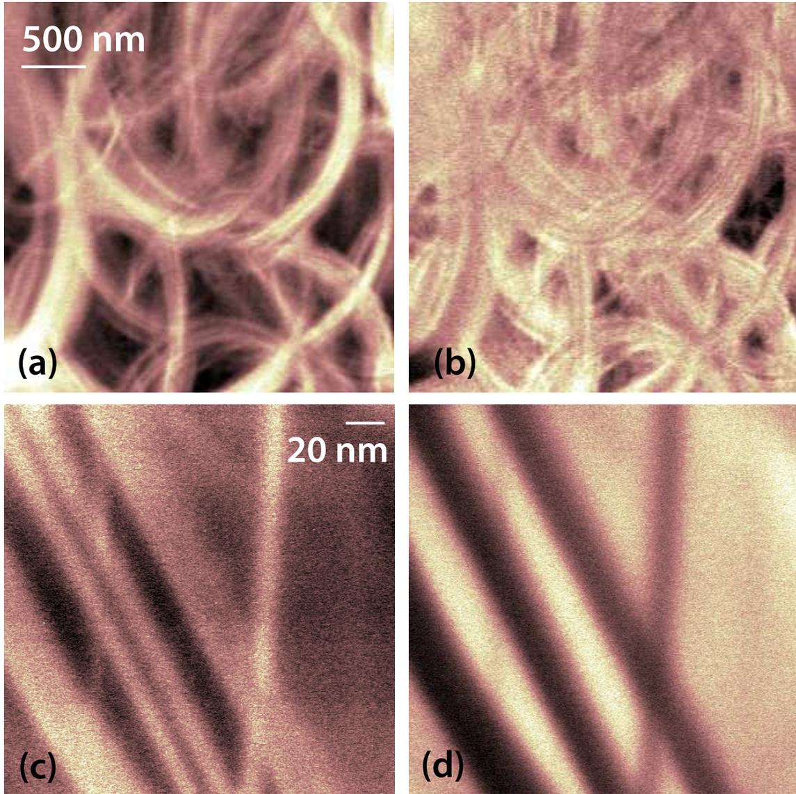
Figure 3-8: (a), (b)  $3 \times 3 \mu\text{m}$  in-phase and lagging phase images taken at  $\nu_{\text{bulk}} = 1.1$  (5.5 T) and  $V_{\text{tip}} = -1.5\text{V}$ . Many narrow oscillations are visible in these arcs in these images. (c), (d) Ultra-high resolution scans ( $200 \times 200 \text{ nm}$ ) showing oscillation structures down to length scales comparable to and smaller than the magnetic length.
