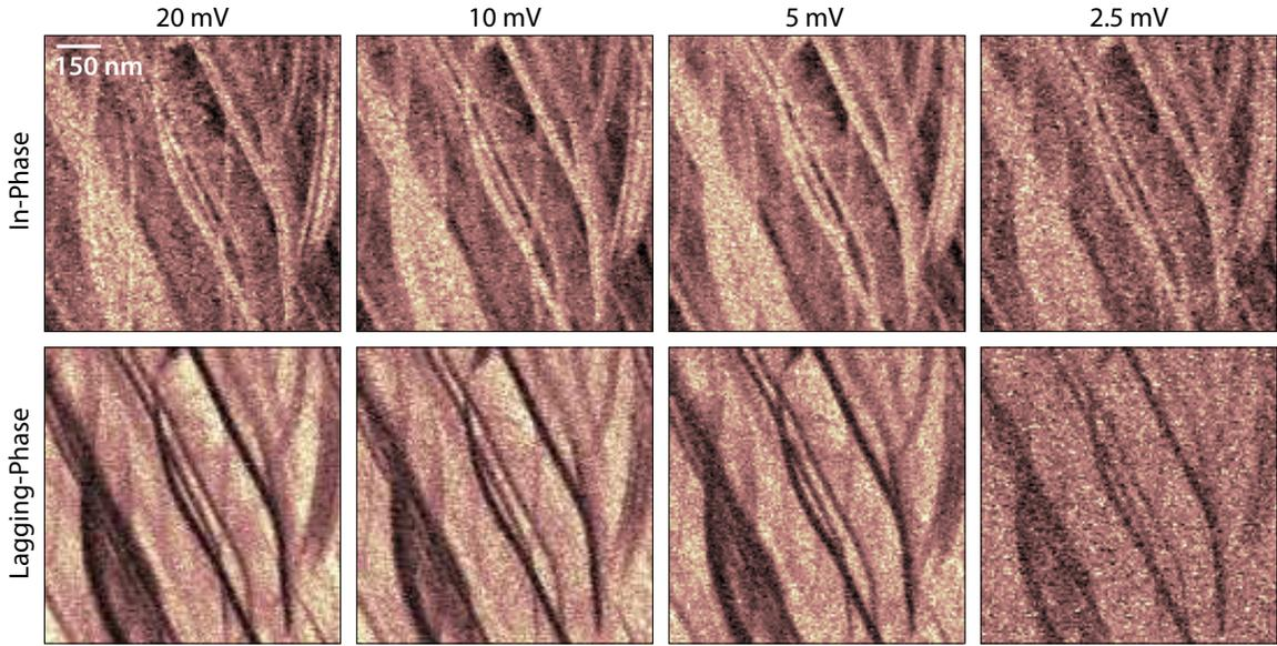
Figure 3-29:  $1 \times 1 \mu\text{m}$  electron bubble images taken at 6.9T ( $\nu = 0.9$ ) with varying excitation amplitudes. For these images, the averaging time at each excitation was the same. These were taken with the same tip as in figure 3-28.
