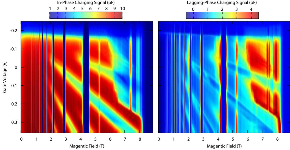
Figure 4-9: In-phase and lagging-phase charging signal after illumination with the LED. After illumination,  $\nu_{\text{bulk}} = 1$  occurs at 9T. The data shows a similar resistive suppression of the charging signal at low bias voltage on the low-field side of integer filling factors in the bulk as shown in figure 4-7.
