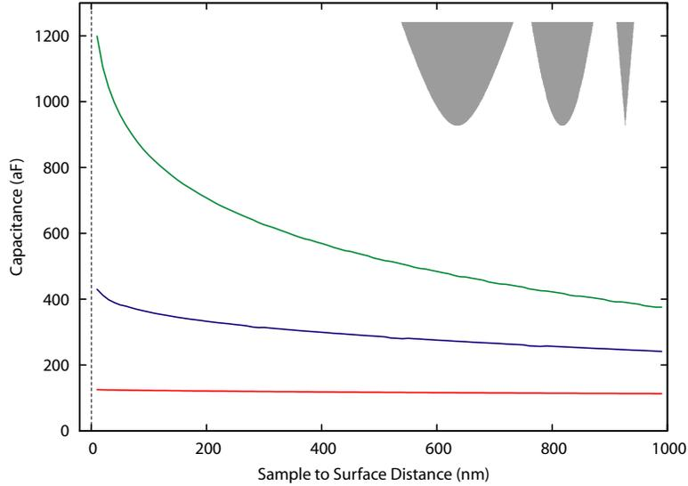
Figure 5-8: Calculated approach curves for different shaped tip, shown at the top right. The curve from figure 5-7 with a pitch of 1.6 and a radius of  $5 \mu\text{m}$  is shown in green. Increasing the tip pitch to 10 with the same radius, shown in blue, decreases the magnitude of the upturn. The curve for a perfectly sharp tip (10 nm) is shown in red. This curve shows no “upturn” at all.
