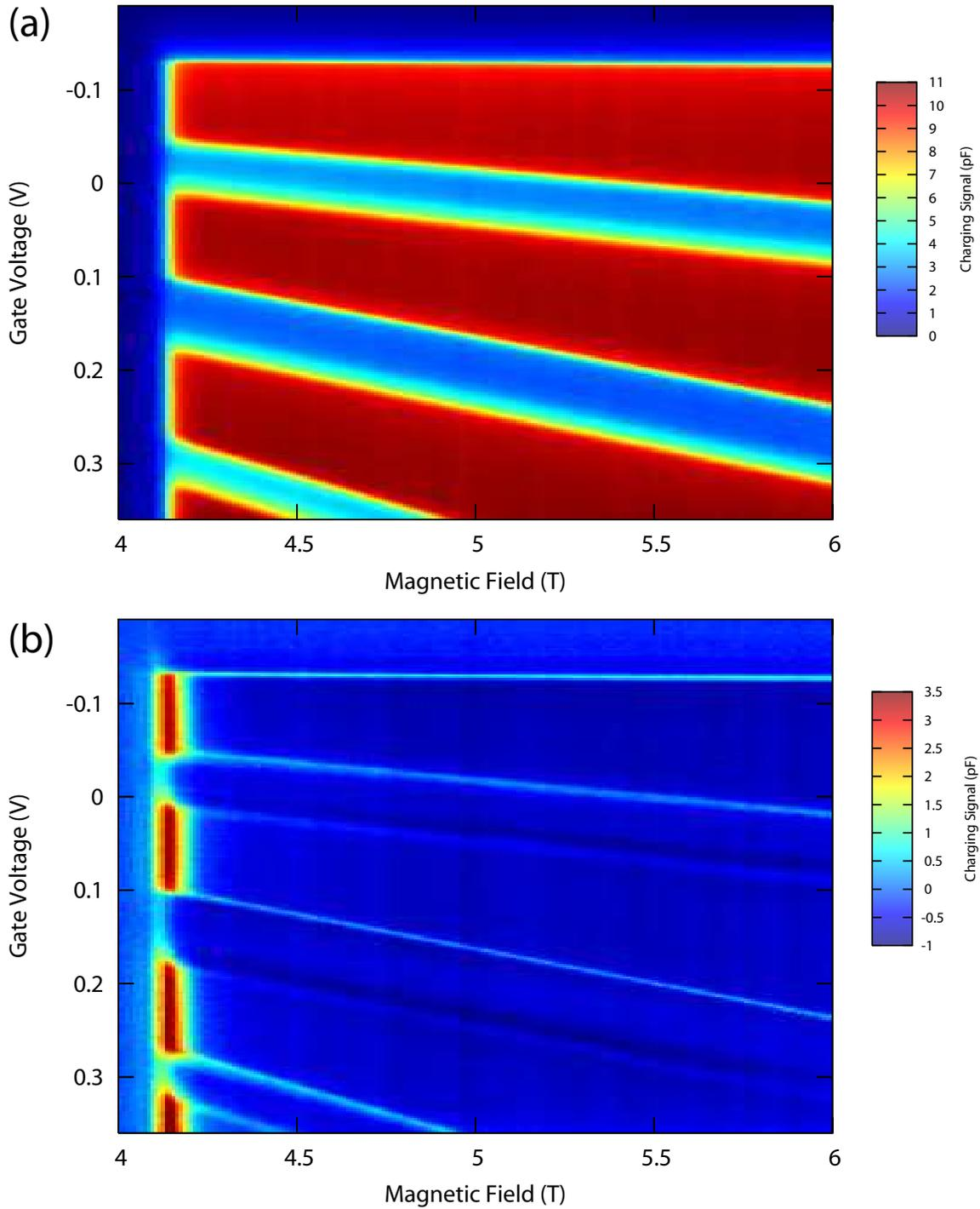
Figure 4-4: In-phase (a) and lagging-phase (b) data taken at 1 kHz. Remarkably, for  $\nu_{\text{bulk}} < 1$  ( $B > 4.2\text{T}$ ), the lagging phase signal is very small in magnitude when the bias voltage is swept so that the local area under the pad is at integer filling. This small lagging phase signal implies that the large drop seen in the in-phase signal contains a significant contribution from the density of states.
