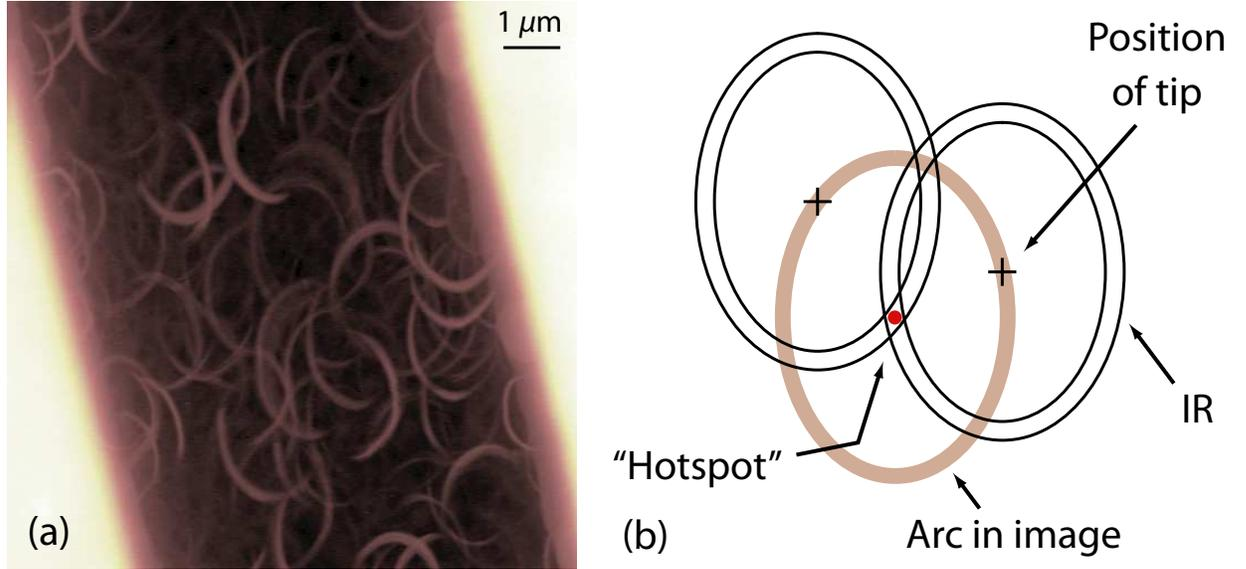
Figure 3-5: (a) A  $10 \times 10 \mu\text{m}$  in-phase charging image taken at  $\nu_{\text{bulk}} = 0.89$  ( $B = 7.0\text{T}$ ) with a bias of  $+1.5\text{V}$  applied to the tip. The image is generally dark, but is penetrated by bright arcs at positions where the IR becomes leaky. (b) Intersection of the IR with hotspot of fixed position in the 2DES creates the arc patterns shown in the image in (a) that reproduce the shape of the IR inverted through the hotspot.
