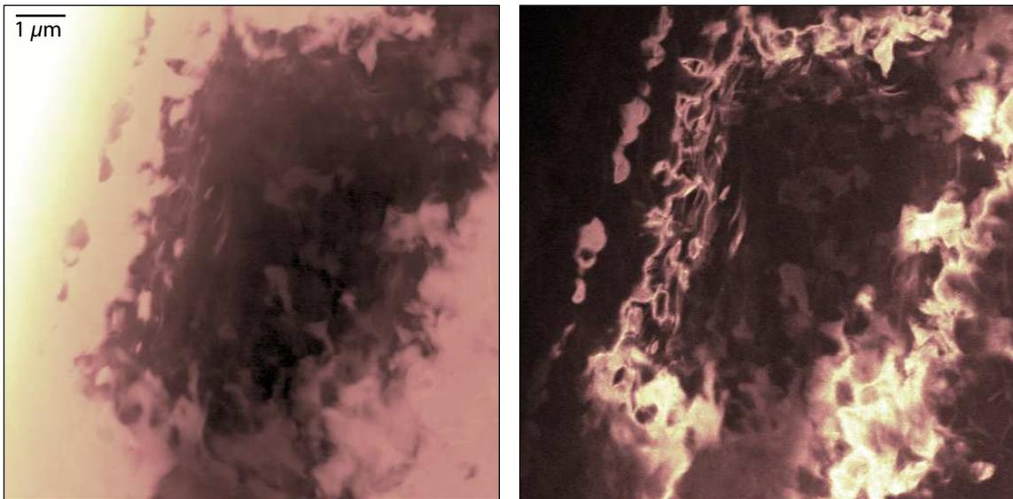
Figure C-7:  $10 \times 10 \mu\text{m}$  in-phase and lagging phase images at 6.4T and 0.25V (near null) with a 10 mV excitation. Compared to the 5 mV images, the sharp edges are smeared slightly, although they are still much sharper than the electrostatic resolution.
