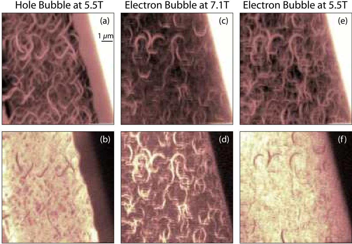
Figure 3-12: Comparing electron and hole bubble images at the same magnetic field. (a),(b) In-phase and lagging-phase hole bubble images at 5.5T at an electron density of  $1.5 \times 10^{11} \text{ cm}^{-2}$ . (c), (d) Electron bubble images at 7.12T at the same density. In (e) and (f), the sample density was lowered to  $1.16 \times 10^{11} \text{ cm}^{-2}$  to allow electron bubble images to be taken at the same magnetic field as the hole bubble images in (a) and (b).
