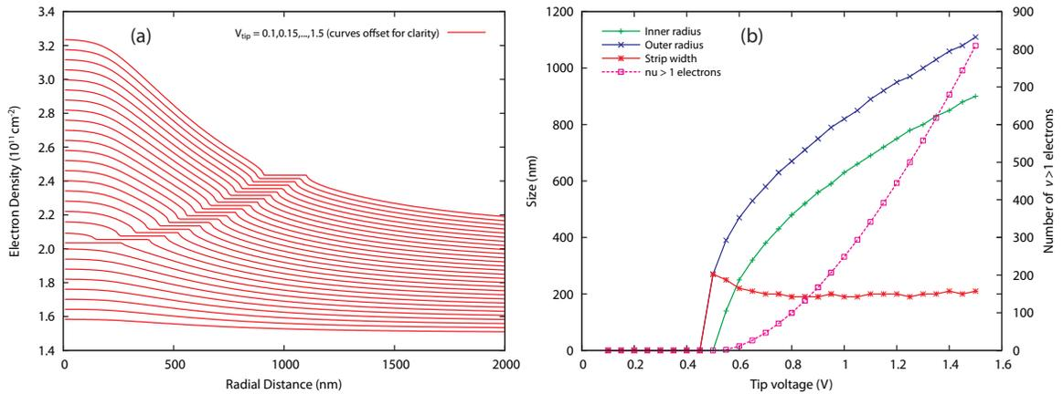
Figure 5-10: (a) Density profile at a magnetic field corresponding to  $\nu_{\text{bulk}} = 0.8$  with increasing bias voltage applied to the tip showing the formation of the IR. (b) The dimensions of the IR and the occupation of the central bubble as a function of tip bias voltage. The calculations were performed for a tip with  $r = 5 \mu\text{m}$  and a pitch of 1.6.
