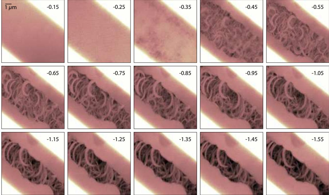
Figure 3-14: A sequence of images from a hole-bubble bias sweep. The  $10 \times 10 \mu\text{m}$  images show the in-phase charging signal at 5.5T for the tip bias voltage indicated in the top right of the images.
