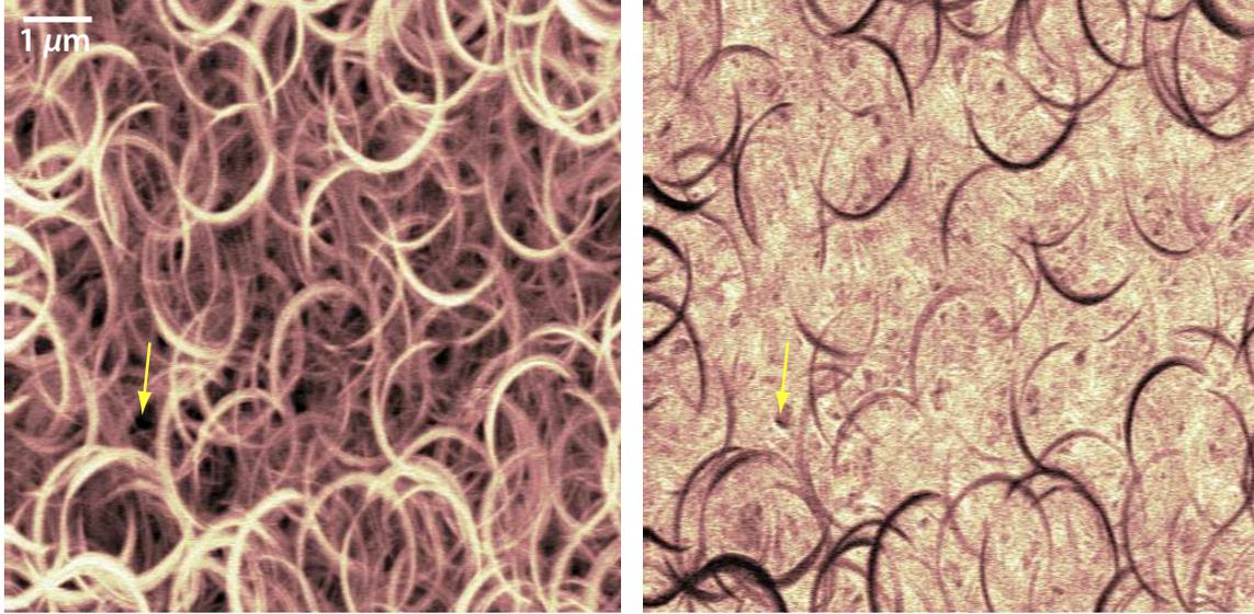
Figure 3-11:  $9 \times 9 \mu\text{m}$  high resolution hole bubble images. Hole bubble images display a spectacular tangle of arcs, implying a very high density of active hotspots. Arrows denote a place in the image where the IR does not intersect any hotspots. The IR has a high resistance at this position, producing a dark signal in both the in-phase and lagging-phase images.
