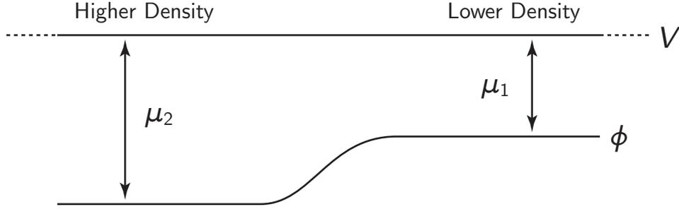
Figure 5-2: A semiconductor held at electrochemical potential  $V$  where the electron density is varying with position. The chemical potential  $\mu$  is larger in regions of higher density. In order to maintain a constant electrochemical potential  $V = \phi + e\mu$ , the electrostatic potential  $\phi$  must drop.
