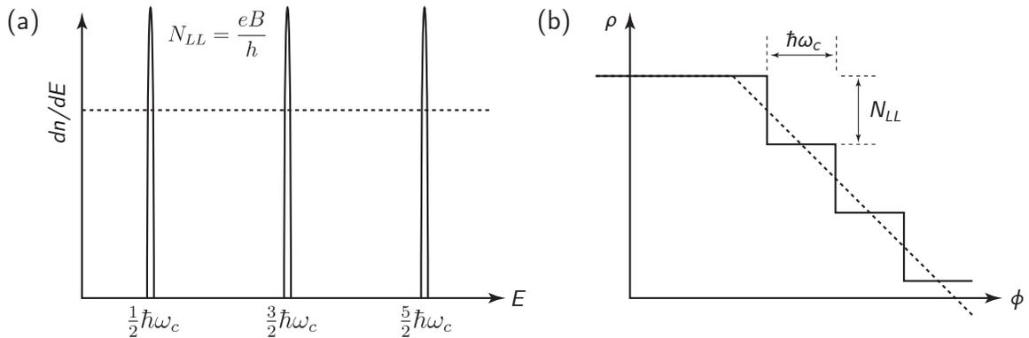
Figure 5-4: (a) In a magnetic field, the zero field density of states (dashed) breaks into  $\delta$  functions separated by  $\hbar\omega_c$ . Each Landau level holds  $eB/m$  electrons, resulting in a staircase  $\rho(\phi)$  shown in (b) that follows the slope of given by the zero field density of states (dashed).
