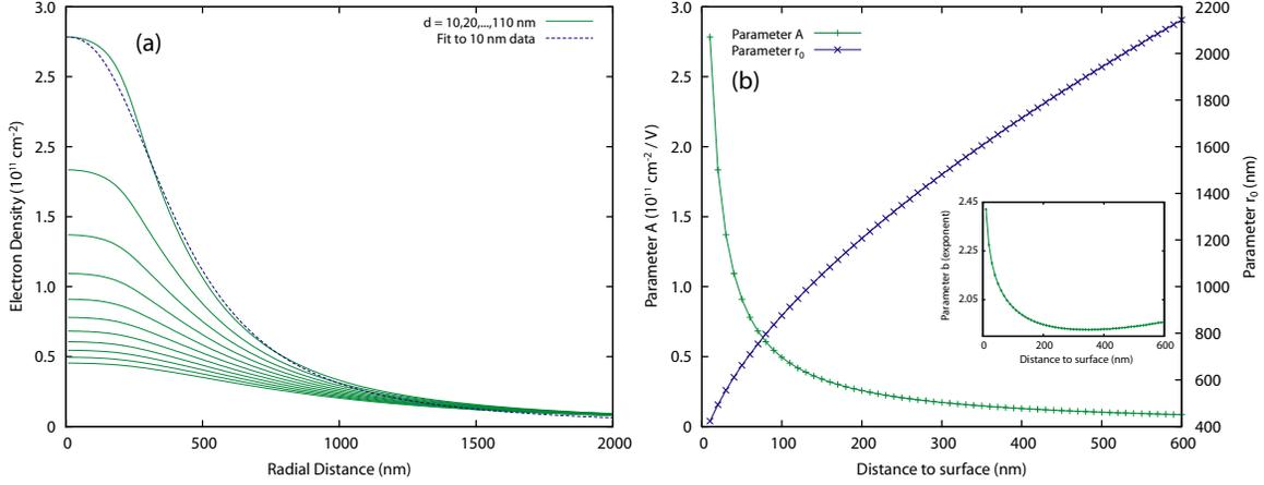
Figure 5-14: (a) Green lines show the density profile for a voltage of 1V applied to the tip at different distances  $d$  from the surface. The blue dashed line shows the fit to equation 5.10 for a 10 nm distance from the surface. (b) Parameters obtained from fitting the density profile at different sample-tip separations.
