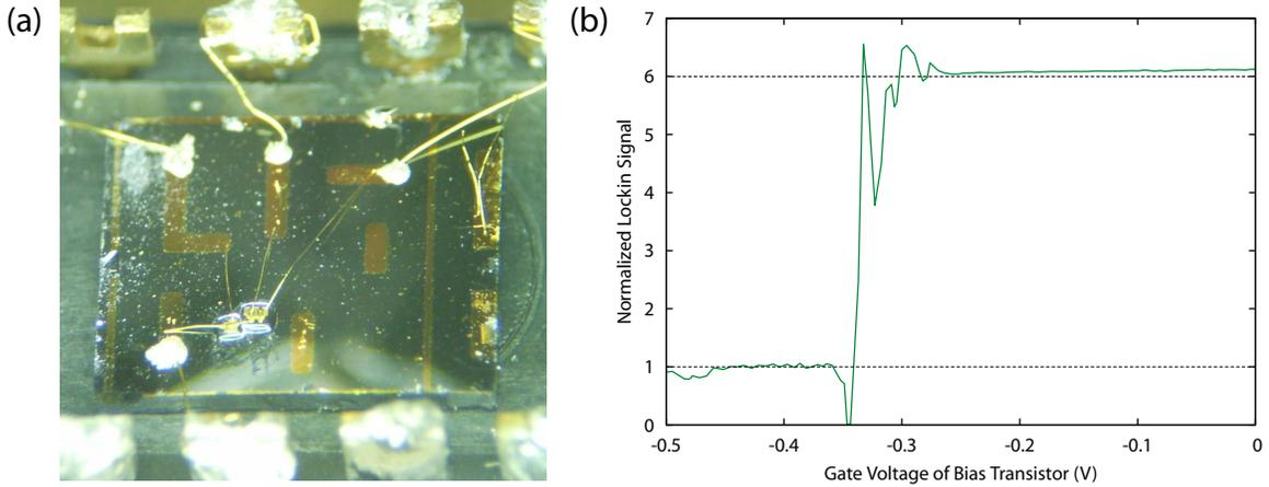
Figure A-3: (a) The transistor setup used to measure the minimum possible center point bridge capacitance  $C_T$ . (b) A pinch off measurement to determine the ratio of the  $C_T$  to the bias transistor source-drain capacitance. The measurement shows that the minimum possible capacitance is about 600 fF. The mount fabrication and capacitance measurement was performed by Eric Lin.
